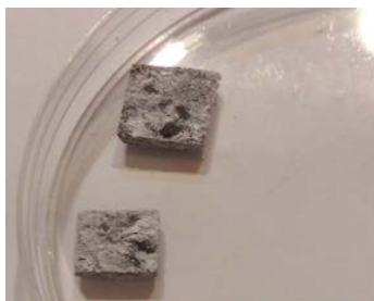
Om deposition of HA on Bamboo charcoal
